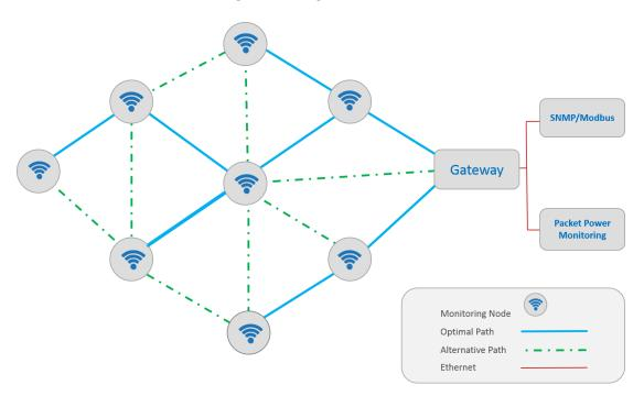
The Packet Power network utilizes **dynamic routing**. Each time a device transmits, it evaluates the performance of the network paths through all the other monitoring units it can communicate with, determines the optimal network path, and makes a short data transmission.
