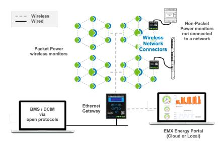
Connect the Wireless Network Connector (WNC) into the Ethernet or serial port of a supported device and connect the WNC's power supply. The WNC recognizes the connected device and immediately begins to send data across Packet Power's wireless mesh network similar to other Packet Power wireless monitors.
